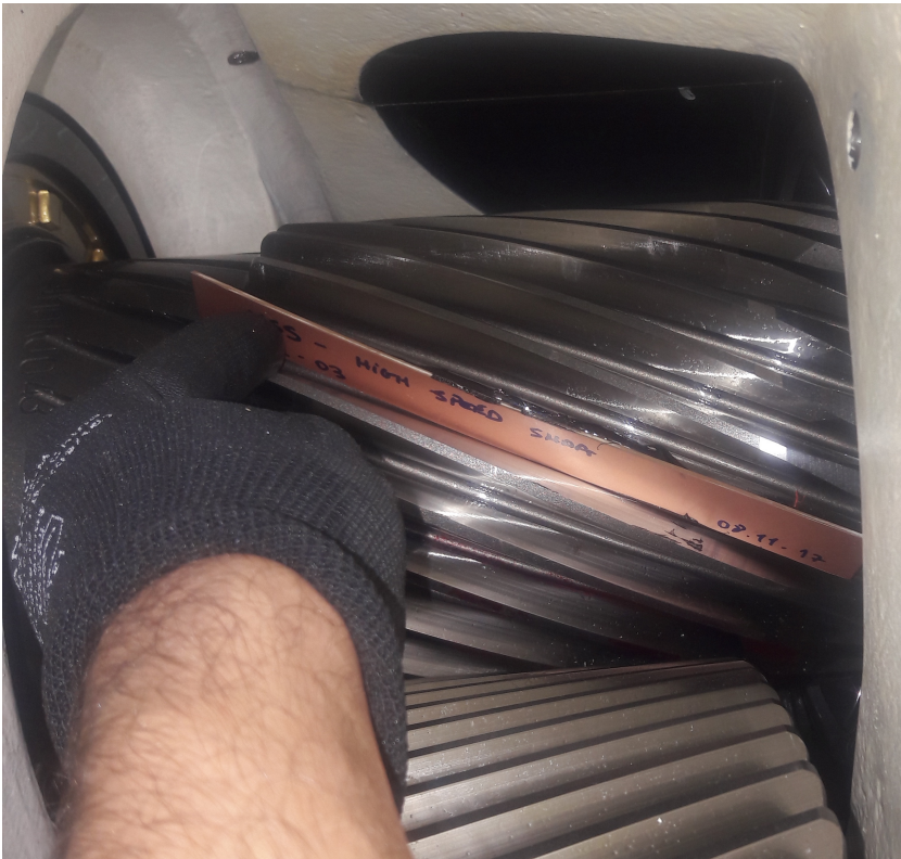
Image 6: Surface imprints of a tooth flank of the HSS were taken on 08.11.2017
