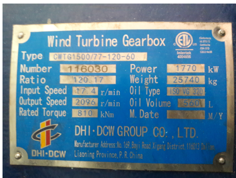
Image 2: name plate of BC-03gearbox
