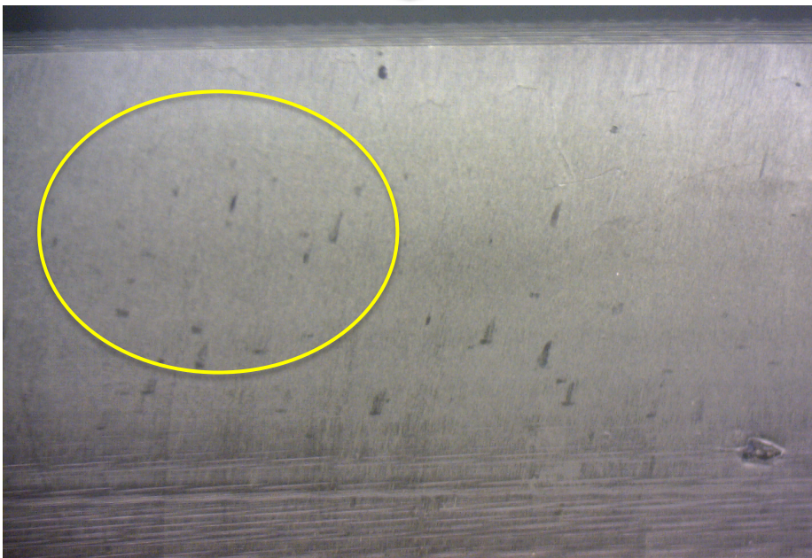
Image 10: BC-03 HSS after the REWITEC ® surface treatment on 09.01.2018
