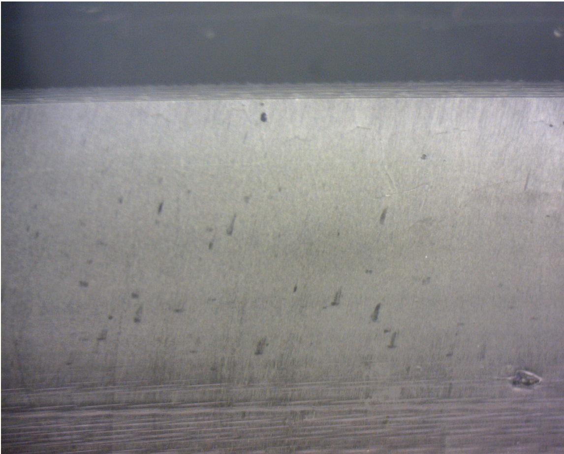
Image 10: Surface imprint of BC-03 HSS after the REWITEC ® surface treatment on 09.01.2018
