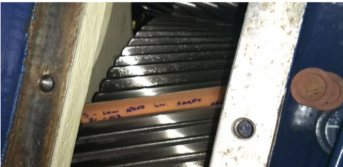
Image 5: Surface imprints of a tooth flank of the LSIS were taken on 08.11.2017
